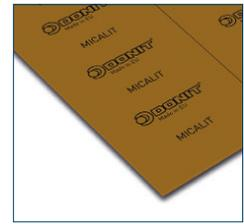
MICALIT<sup>®</sup> P is mica based material with tanged stainless steel insert. It has excellent thermal, good chemical and mechanical resistance making it suited to the high temperature conditions of the automotive and steel industry, exhaust systems, burners and ovens. It has good electrical insulation and low thermal conductivity properties.
